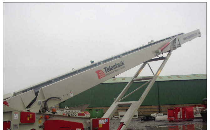
Heavy duty - 21 metre (70ft) Incline conveyor
