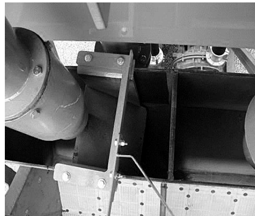
Movable chute to allocate fine material to the coarse product
