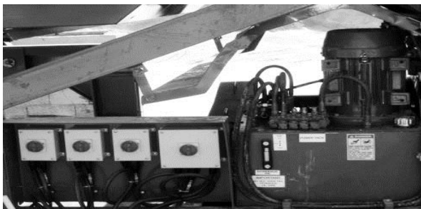
Integrated electric powerpack for bucket wheel speed adjustment
