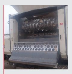
Medium speed shredder with aggressive cutting teeth
