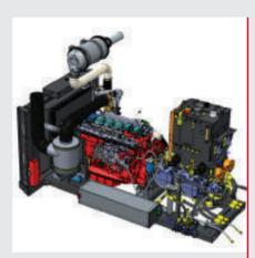
A powerful Scania engine with a low operating speed combined with an efficient hydrostatic drive creates a very responsive shredding action with protection against unshreddable contaminants
