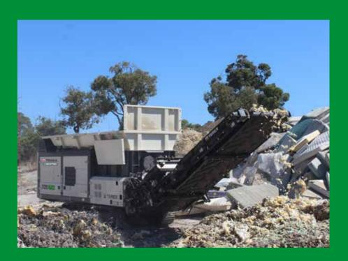
Key features include the hydrostatic drive offering better protection against contamination and allowing for bi-directional shredding. The double shaft shredder has 2m long shafts with a fully welded tooth configuration, impressive throughput and excellent reduction.
