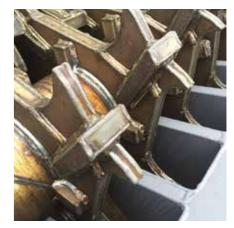
Shaft cutting elements are a fully welded structure with hard-faced edges giving ultimate strength in difficult applications
